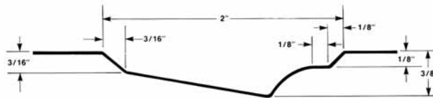
ENTRY DOOR TYPICAL PROFILE
